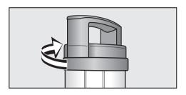
To rinse the milk pipework: Fill the larger of the two plastic containers to the "max" mark with **cold** water. Make sure that the lid of the stainless steel milk flask engages properly.
